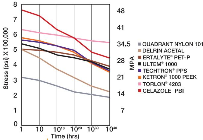
Fig.3 - **CREEP AT 300°F (150°C) - ISOMETRIC STRESS - TIME CURVES**
